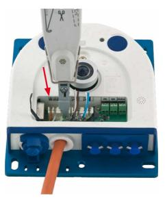
If additional cables are required inside the housing (MxBus, microphone, speaker), they must be connected as described in *Section 2.5.3, «Connecting Additional Cables».*
