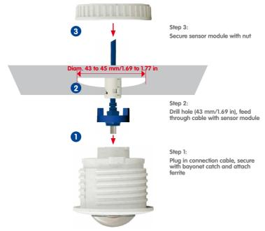
It should be ensured when selecting installation sites that each of the sensor cables do not exceed 2 m/6.6 ft. The theoretical maximum distance between the two sensor modules of a S15D where the base module is placed centrally is therefore 4 m/13.1 ft.
