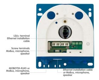
Before laying the Ethernet installation cable, remove the bayonet catch and replace the Ethernet patch cable plug with either one of the additional plugs (M.4/5) or the single wire plug (2.10), depending on the cable used.
