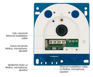
Before laying the Ethernet installation cable, remove the bayonet catch and replace the Ethernet patch cable plug with either one of the additional plugs (M.4/5) or the single wire plug (1.8), depending on the cable used.
