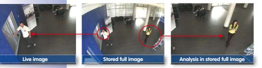
Stored full image: Original camera image without distortion or image correction This means that you can use the vPTZ features in VGA resolution to pan, tilt and zoom in the live image while the camera is, for example, recording full images at 1 fps in MEGA or QXGA resolution.
