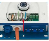
Ensure that the installation cable is fed right into the housing when the camera is in the right position so that the cable plug provides optimal sealing for the housing
