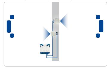
In L-shaped rooms, both sensor modules are simply positioned at right angles. A S15D therefore captures the entire room without any blind spots.
