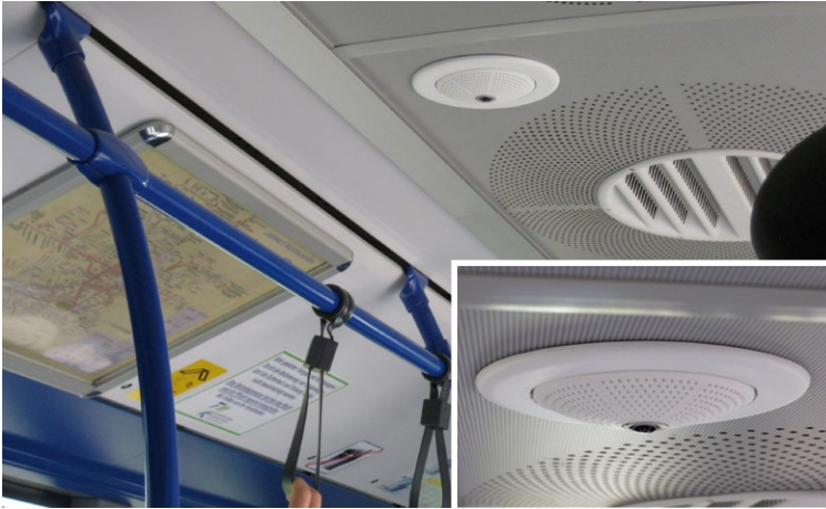
Q25M in the In-Ceiling Set (local public transport bus)
